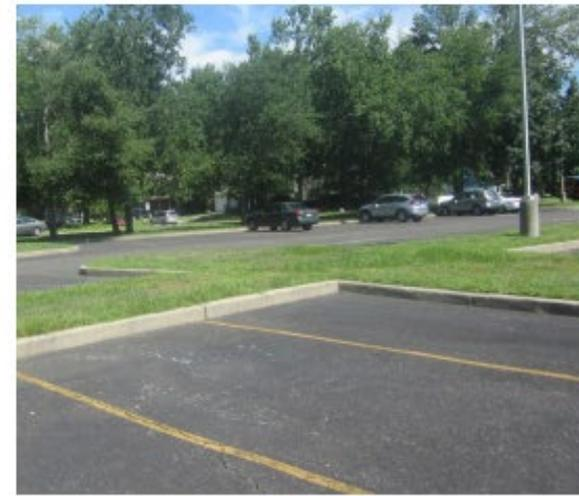
Stormwater is currently directed to an existing catch basin. Installing rain gardens in the parking lot islands can capture, treat, and infiltrate stormwater runoff from the parking lot. Replacing parking spaces with porous pavement can capture and infiltrate runoff from the other side of the parking lot. A preliminary soil assessment suggests that more soil testing would be required before determining the soil's suitability for green infrastructure.
